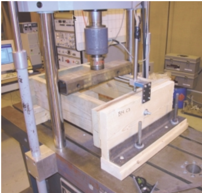
Figure 2. The hydraulic test machine put pressure on a pair of joists attached by hangers to the sample ledger (above). Extra fasteners in the hangers ensured that failure would occur not at the hanger but in the lag screw or bolt attaching the sample ledger to the sample band joist. A transducer measured displacement of the ledger (above right), while a computer continuously recorded measurement and load data. The load was applied until the connection failed (right).
