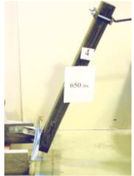
Figure 5. The authors tested the HD2A connection with the post installed both inside and outside the band joist; both configurations withstood the full test load. At 200 pounds, the sample post shown above deflected but the connection held; at 650 pounds, with the post still holding, the test was ended so as not to damage the test machine.
